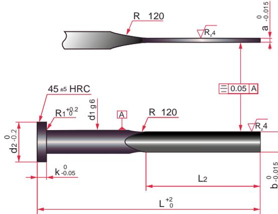
Mat.: 1.2210 / 58±2 HRC. DIN 1530A / Dureza recubrimiento > 70 HRC. Maximum temperature at work: 220° C
